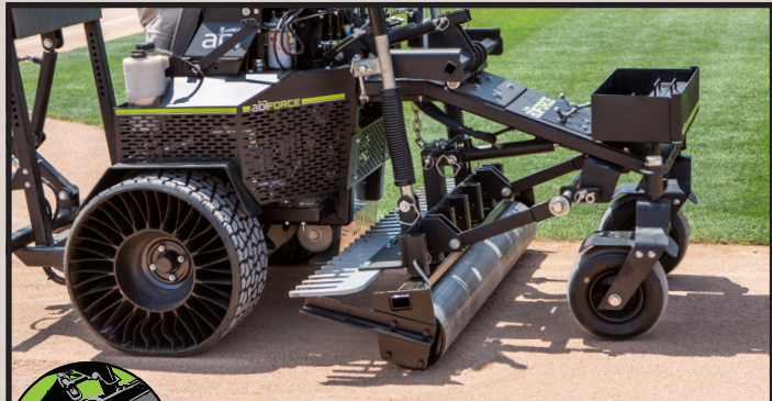
ROLLER W/WEIGHTS 58" WIDE, APPROX. 1/2 TON PRESSURE
