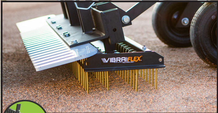
VIBRAFLEX 3800 60" WIDE | 3/4" SPACING | 1/4" OR 3/8" PINS
